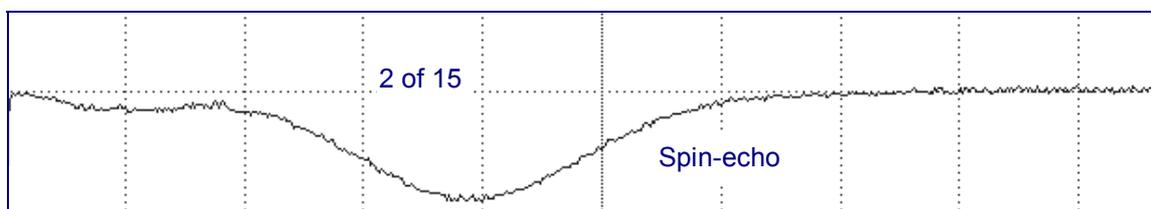
We are interested in determining the relative max amplitude of the acquired FID signals at the same time the pulse.
