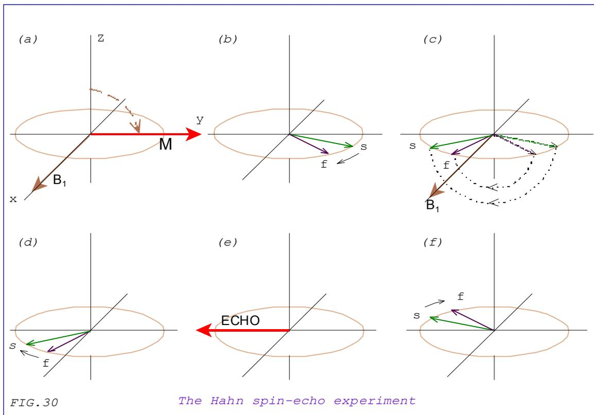
If the steady magnetic field were perfectly homogeneous, the echo amplitude might be just as large as the initial FID following the  $90^\circ$  pulse. However, the magnetic moment vectors lose phase coherence not only because of field inhomogeneities, but also because of the inherent processes responsible for transverse relaxation. These “natural” processes, however, are irreversible and cannot be refocused.
