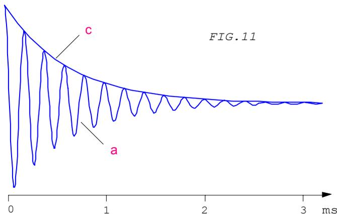
The signal decay parameters characterise the sample. Fig.11 shows a comparison of two signals, a and c, in Fig.10. The amplitudes of the signals decay simultaneously towards zero with a time that depends on the sample under investigation. (For the glycerine sample this time is ~ 3ms).
