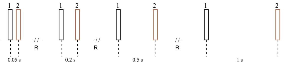
The sequence can be written as  $90^\circ - 0.05s - 90^\circ - R - 90^\circ - 0.2s - 90^\circ - R - 90^\circ - 0.5s - 90^\circ - R - \dots$
