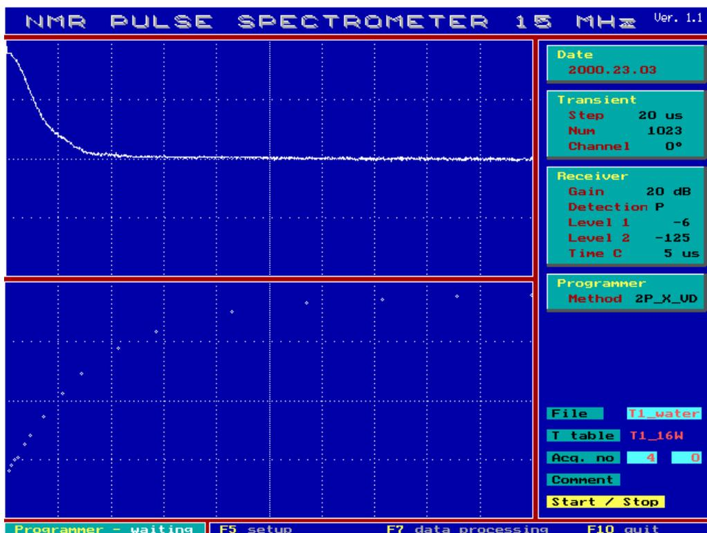
When running the Acquisition mode the user performs an experiment with signal storage in a binary file. The screen is divided into two viewing windows. The upper window is used for presentation of the real-time run NMR signals and the bottom window to show signals current amplitudes versus delay according to Variable Delay (VD) table. This is useful function during  $T_1$  and  $T_2$  measurements (See Practical Considerations in  $T_1$  and  $T_2$  experiment).
