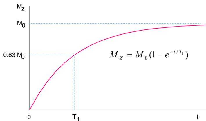
$T_1$  is the time for the longitudinal magnetization,  $M_z$ , to recover from 0 to  $(1 - e^{-1})$  or about 63% of its final value  $M_0$ . In the literature, the  $T_1$  relaxation curve is usually plotted in a semi-logarithmic diagram, i.e., with logarithmic values along the ordinate (y-axis) and time along the abscissa (x-
