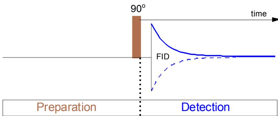
**Preparation includes of instrument setting and sample. During preparation the spin system of the sample is set to a define state. The latter is determined by a delay between repeat scans (Recycle delay) to allow relaxation; that is, the return of the macroscopic magnetization  $M_0$  to the z-axis after the previous pulse and before the next pulse is applied.**
