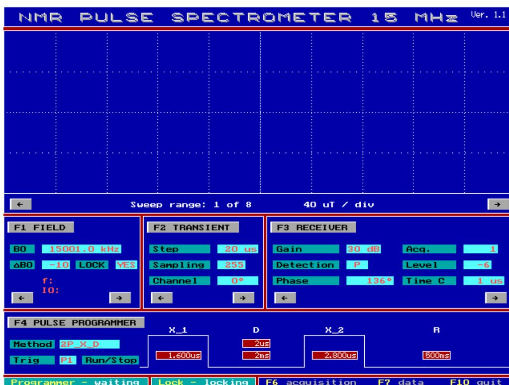
The program opens the Setup screen (F5) and starts the NMR measurements after the completion of the automatically adjusting and stabilizing the magnetic field  $B_0$ .
