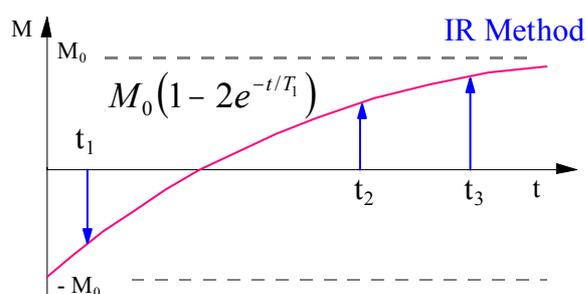
To determine  $T_1$  via the  $180^\circ$  -  $t$  -  $90^\circ$  sequence (IR method),  $\mathbf{M}$  is inverted by a  $180^\circ$  pulse at  $t = 0$ . After a delay of  $t$  seconds a  $90^\circ$  pulse sampling pulse is used to monitor the recovery of  $\mathbf{M}$ . (In the PS-15 select the “M2\_90X” in the method list to perform the IR sequence).
