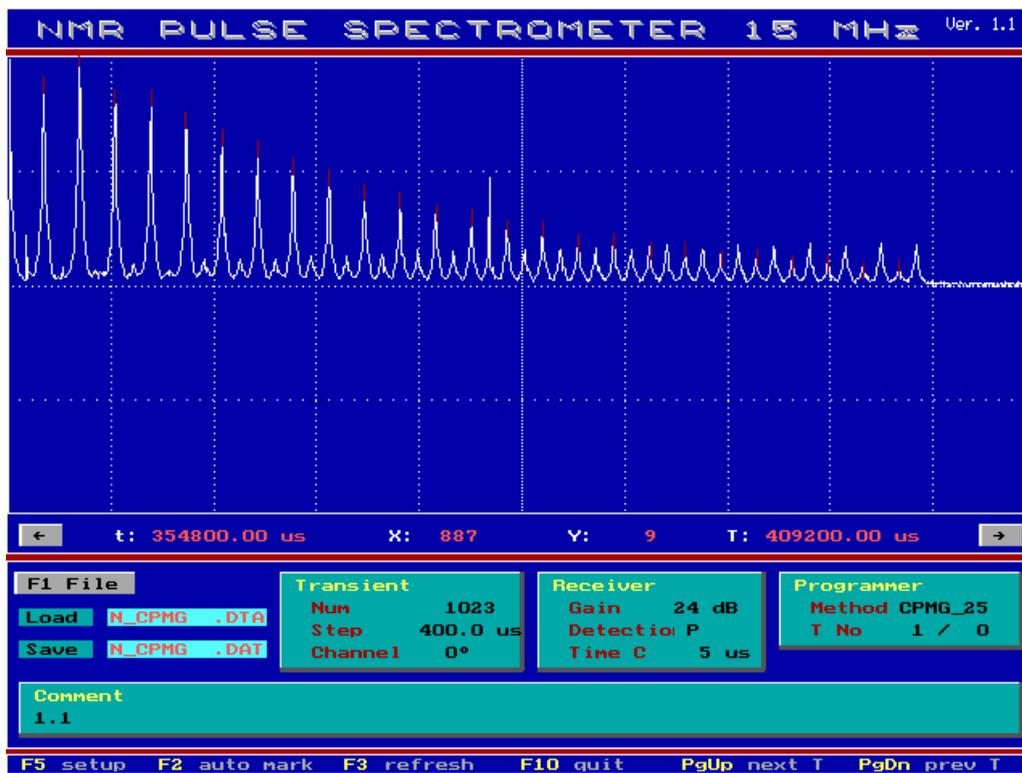
The created file consists of two columns; time vs corresponding magnitude of the echo signal. An example is shown in Fig.37 (data points obtained from the spectrum in Fig.36).
