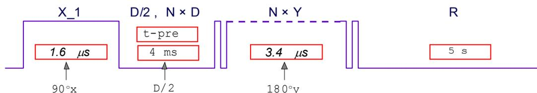
The system repeats the measurements with the recycle delay  $R$  (In the figure  $R = 5$  s). It is also the separation period between the runs while a multi-scanning spectral superposition capability of the system is used. That is, when the  $\langle \text{Acq.no} \rangle$  is set larger than 1 in the F6 acquisition mode. A multi-scanning option is particularly useful for the samples with a weak signal. The recycle delay should be set at least five times  $T_1$ .
