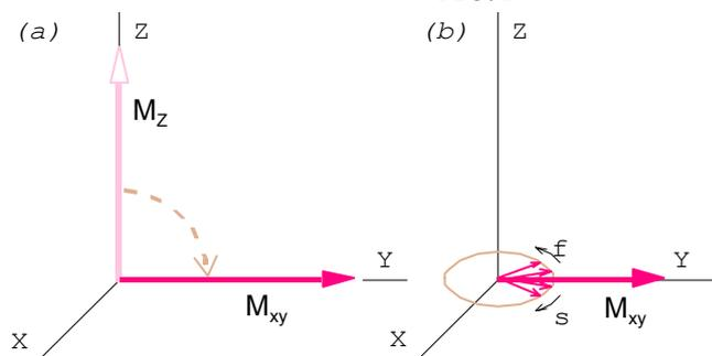
Fig.28 illustrates the dephasing of the proton magnetic moments causing  $T_2^*$  decay (see Fig.26) of the transverse magnetization, depicted
