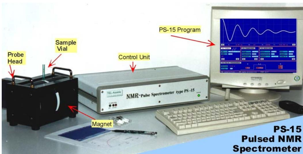
*PS-15 is not only easy to use, it is easy to understand since each module has its own clearly defined function in the spectrometer and is accessible to individual examination with the computer keyboard.*
